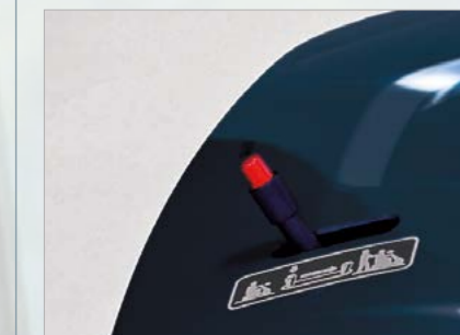
Two-step disengaging lever to prevent free-wheeling
